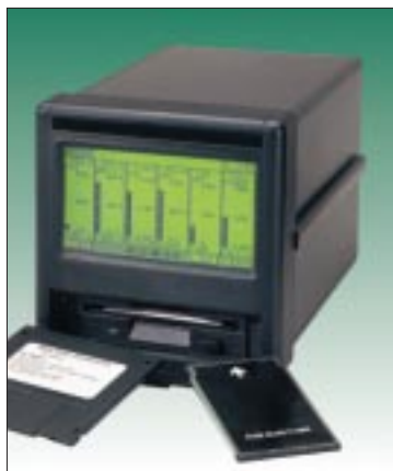
Magnetic storage media, on PCMCIA card or floppy disk, allow videographic recorders to download data for archival storage.
